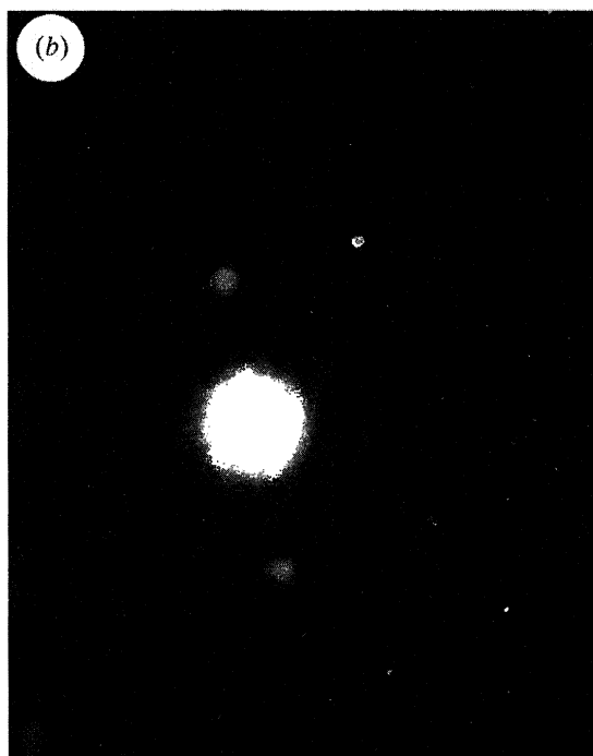
Figure 7. Triple 30°-bent nanotube and SAEDP are shown. The patterns in regions (a) and (b) show that helicity changes by 30° after and before the bend. This may imply a change in the electronic structure due to the insertion of the pentagon–heptagon pair.
